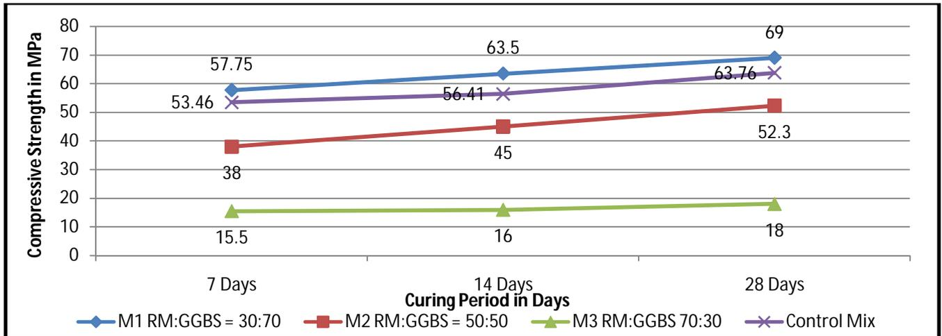
Graph 2: Compressive strength of cubes subjected to ambient curing
